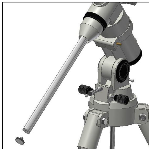
Figure 15. Remove foot saver to slide Counter-weight.
