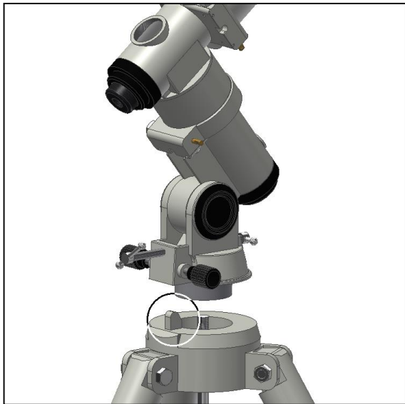
Figure 13. Align mount and tripod post.
